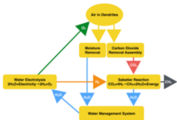
Figure 3.2.1-1 ISS Oxygen Generator System
