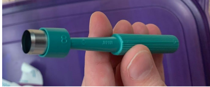
Figure 3. Harris Uni-core 8 mm diameter puncher provided by Professor Fu’s lab team. The 8 mm model is used to create ports that connect to the cell loading and induction channel, as shown in Figure 1, pg. 6. The 1.2 mm puncher was not provided so no image is available.
